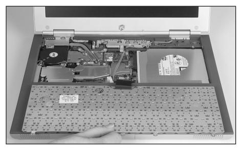
10 Disconnect the keyboard by lifting the keyboard connector using two fingers. Be careful to not touch or damage any other components.
