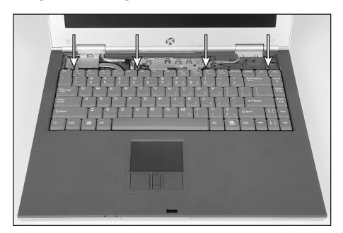
Remove the keyboard by raising the back edge, then slowly rotating it toward you so it lies **keys-down** on top of the notebook. Be careful not to damage the LCD panel.
