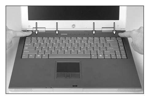
The bezel is correctly mounted when you can run you finger along the bezel and find no loose spots. The bezel should be flat all the way across. If the bezel is mounted incorrectly, complete the instructions under "Replacing the bezel" on page 12.
